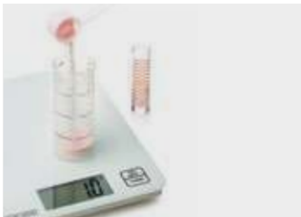
7. Weigh the resin, measure the monomer and mix, pouring the monomer in first and then the resin
