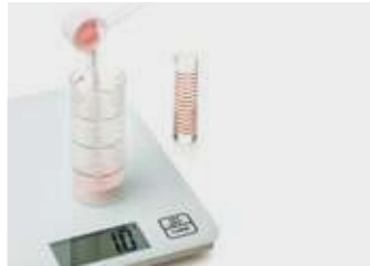
6. Weigh the resin, measure the monomer and mix, pouring the monomer in first and then the resin
