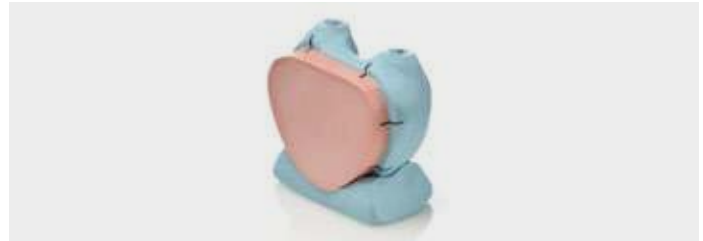
7. Base construction in Platinum 95 to keep the structure in a vertical position, marking of orientation points to check the correct repositioning of the silicone
