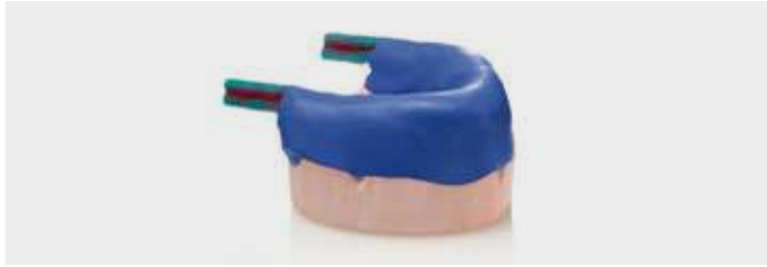
3. Primary mask in Platinum 85 TOUCH, with total coverage of the wax-up (allows superior detail reproduction of the wax-up)
