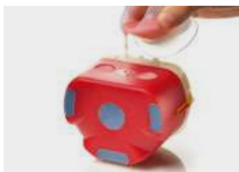
13. The pouring is complete when the resin oozes out of the side channels
