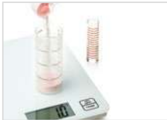
1. Weigh the resin and measure the monomer. Mixing ratio: 10 g of resin and 6.7 g (7 ml) of monomer
