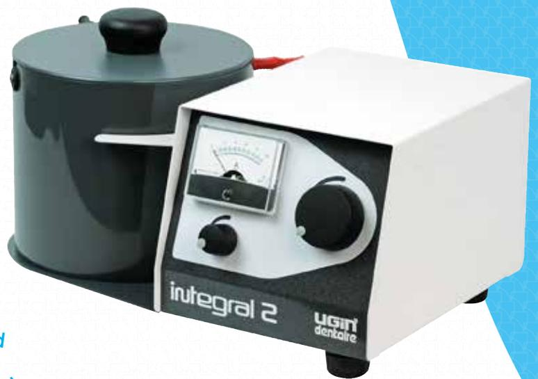
*The **Integral 2** generator uses the principle of electro-substraction. The workpiece is submerged in an acid bath, the high current flowing through it allows a quick and effective polishing (5 to 15 minutes.)*
