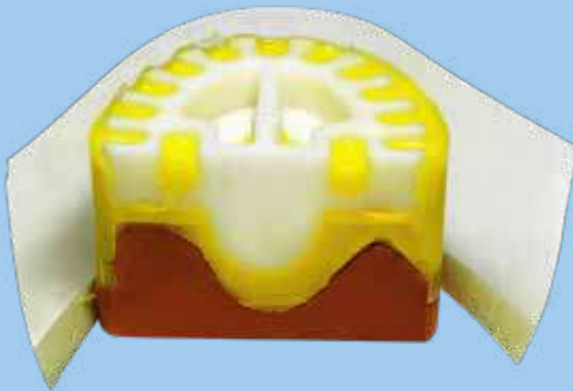
Cross-section of a flaskless duplicating mould
