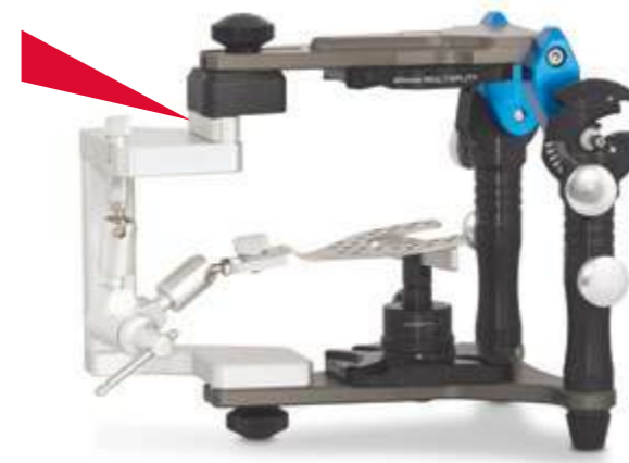
Illustration depicts the transfer carriage #10047 in the Arto articulator with 126 mm construction height. The incisal plate support is swivelled underneath the incisal plate. For a construction height of 116 mm, the incisal plate support is swivelled to the side.
