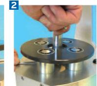
1+2 Unplug the power cable. Insert the fixing pin from the side into one of the holes of the drilling axis. Turn the tubular socket wrench in counter-clockwise direction to unscrew the sleeve nut. Then, remove the defective burr.
