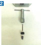
The burr rests on a slotted screw in the center of the axis. Clockwise turns lower the screw = tighter drill hole; counter-clockwise turns raise up the screw = wider drill hole. The wider the drill hole, the farther the pin tip juts out of the plinth plate.
