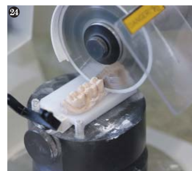
24 Softly hammer on the quadrant plate until the dental arch comes off. Then trim and cut.
